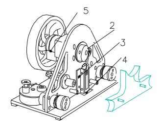
The piezo igniter can be readjusted at two points. 2/3
